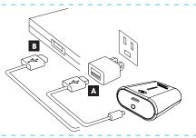
It takes approximately 5-6 hours to fully charge your Pocket Juice Charger (from depleted unit). Once the charging is in progress, the Indicator Lights will illuminate accordingly (see charging chart above).
